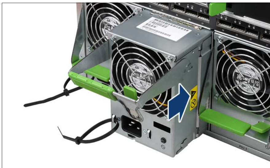
Figure 44: Removing the power supply unit
